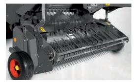
The spiral arrangement of FEED ROTOR tines guarantee even feeding and rapid throughput, while still being gentle on leafy crops like alfalfa. Additionally, the optional pivoting gauge wheels ensure precise ground contour following even at higher speeds or when turning.
