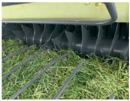
The standard FEED ROTOR on the VARIANT 460 and 480 delivers a uniform crop flow to the bale chamber and is built for rugged performance. All components demonstrate high operational reliability and long service lives, no matter what crops you plan to subject your new VARIANT to in the field. At 540 rpm, high rotor and conveyor speeds are achieved, which in turn accelerates the bale formation process, equaling higher speeds and faster work rates.
