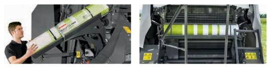
Automatic tying options allow the use of the ROLLATEX net wrap system, twine tying, or both. The new system allows for fast binding, easy loading of the net wrap rolls on the pivoting slide, clear view of the available net wrap from your tractor, and a new net brake for high net tension on the bale.
