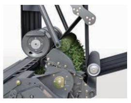
One of the most unique features from the FEED ROTOR or ROTO CUT system, is that the rotor gets the bale turning and forces the bale start – each and every time, under all conditions.
