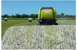
The new extra wide binding comes standard on all 400 Series VARIANT balers. The VARIANT is equipped to operate with 48 inch "Edge to Edge" net wrap or extra wide 51 inch, and transitioning from one size to the other is as simple as moving a few pins. The extra wide provides coverage 2-3 inches over the end of the bale for more secure binding and easier transporting.
