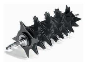
As the hay moves from the pickup into the chamber, it passes through the ROTO CUT knives, which cut the pieces into 2.75 inch lengths. The helical rotor design of ROTO CUT ensures consistent feeding and superior cut.
