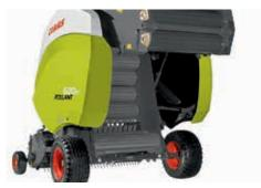
The 17 steel rollers on the ROLLANT 620 were redeveloped to be even stronger and more stable than ever. The internal reinforcement plates strengthen the steel rollers for unsurpassed reliability.
