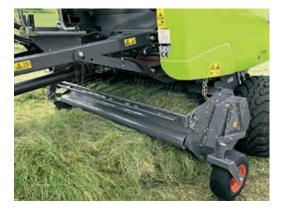
The CLAAS VARIANT was the first round baler on the market with an 83 inch pick-up. This proven design offers enormous throughput capacity. The pick-up is evenly suspended with large caster-mounted guide wheels, keeping it securely on track. This ensures precise following of ground contours and protects the grass stubble, even at high working speeds and when turning.
