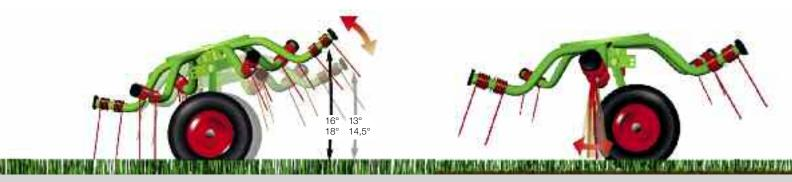
The throw angle can be adjusted quickly and easily. The VOLTO can be set effortlessly for different crops by swapping a bolt position. For use in every crop type - whether there is light or heavy material to be tedded, the tough dual tines take it in their stride.
