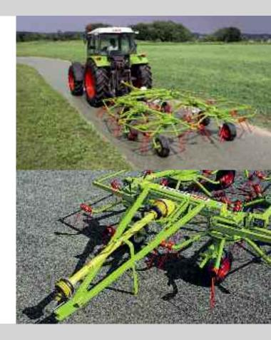
The VOLTO 75 T is fixed to the linkage drawbar or the swinging drawbar. The working height is set with a central crank lever.
