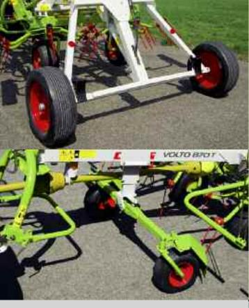
The triangular transport frame and box section chassis provides strength resulting in a long service life.
