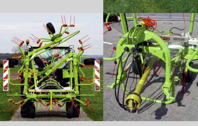
The ingenious folding mechanism on the VOLTO 770 combines its large working width with a low transport height and a close and secure mounting behind the tractor.
