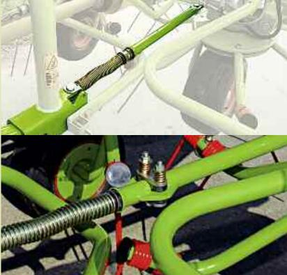
The weight of the tedder is transferred dependably to the robust mounting assembly.
