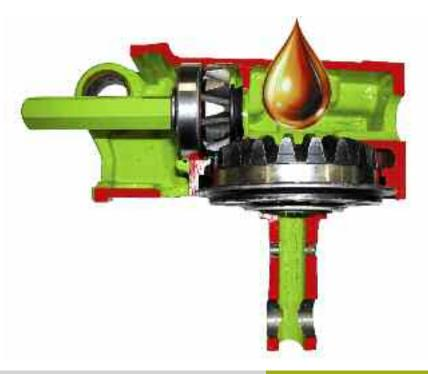
Rotor construction Adhesive grease gearbox
