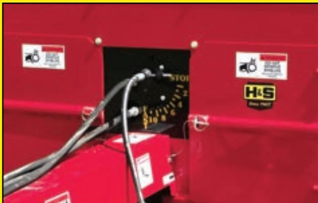
Manual variable speed hydraulic drive available on S3231-SW3243 models
