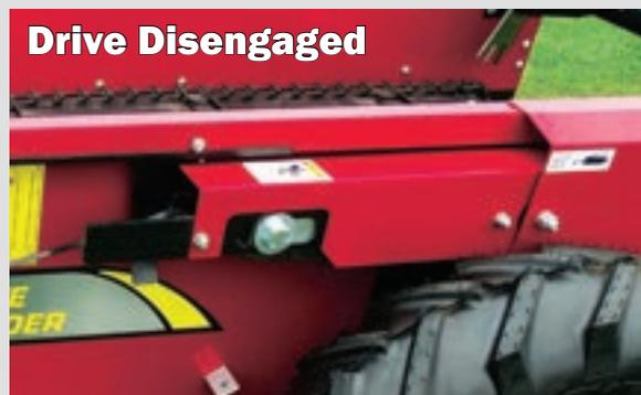
To engage the beater and main apron on the **S1250** and **S1280**, lower the control lever.
