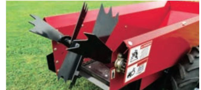
The 20" diameter, 8-paddle beater on the **S1225** provides an even spread of material.
