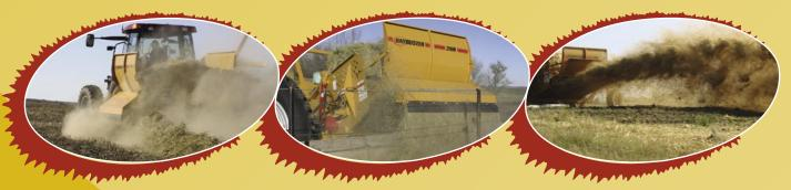
Processing your hay with the 2100 chops the forage into selected cut lengths, mixes drier outside layers with inner, fresher layers, removes dust and molds, and prevents cattle from sorting..... making your hay go farther.
