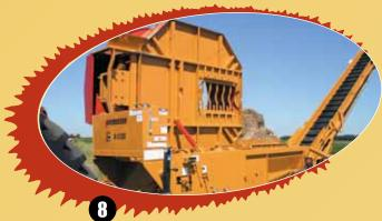
9. The new hydraulic folding 24" (60.96 cm) wide by 26' (7.92 m) long high-capacity stacking conveyor is designed for the increased capacity of the H-1130. A rubber-lagged drive pulley along with Haybuster's "Easy Clean" idler pulley to power the belt. 1<sup>1</sup>/<sub>2</sub>" (3.81 cm) high cleats help haul the ground product away at a high rate without slowing down, even when the hammermill is overloaded. The ground product can be piled up to 18' 6" (5.64 m) high with the conveyor.
