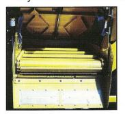
Chain Discharge Conveyor is available for faster unloading of high moisture and high roughage rations.
