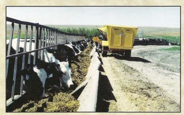
Wide and high delivery door allows easy unloading of mixed ration. Pictured is the 379 Kwikcutter feeding a total hay mixed ration to a dairy herd.
