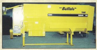
Stationary units allow permanent installation, such as for a feed processing operation or in dairy.
