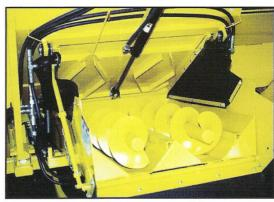
Hydraulically-driven auger discharge for less maintenance and smoother feed delivery.
