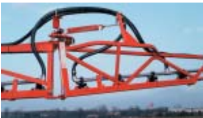
Breakaway wings automatically return to operating position
