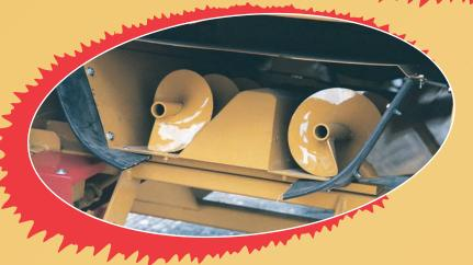
The two heavy-duty and high capacity augers mounted in the **belly pan**, convey the product to the discharge conveyor. The auger and pan combination provides for a high-speed transfer of the product and for a clean, leak-free environment under the tub grinder.
